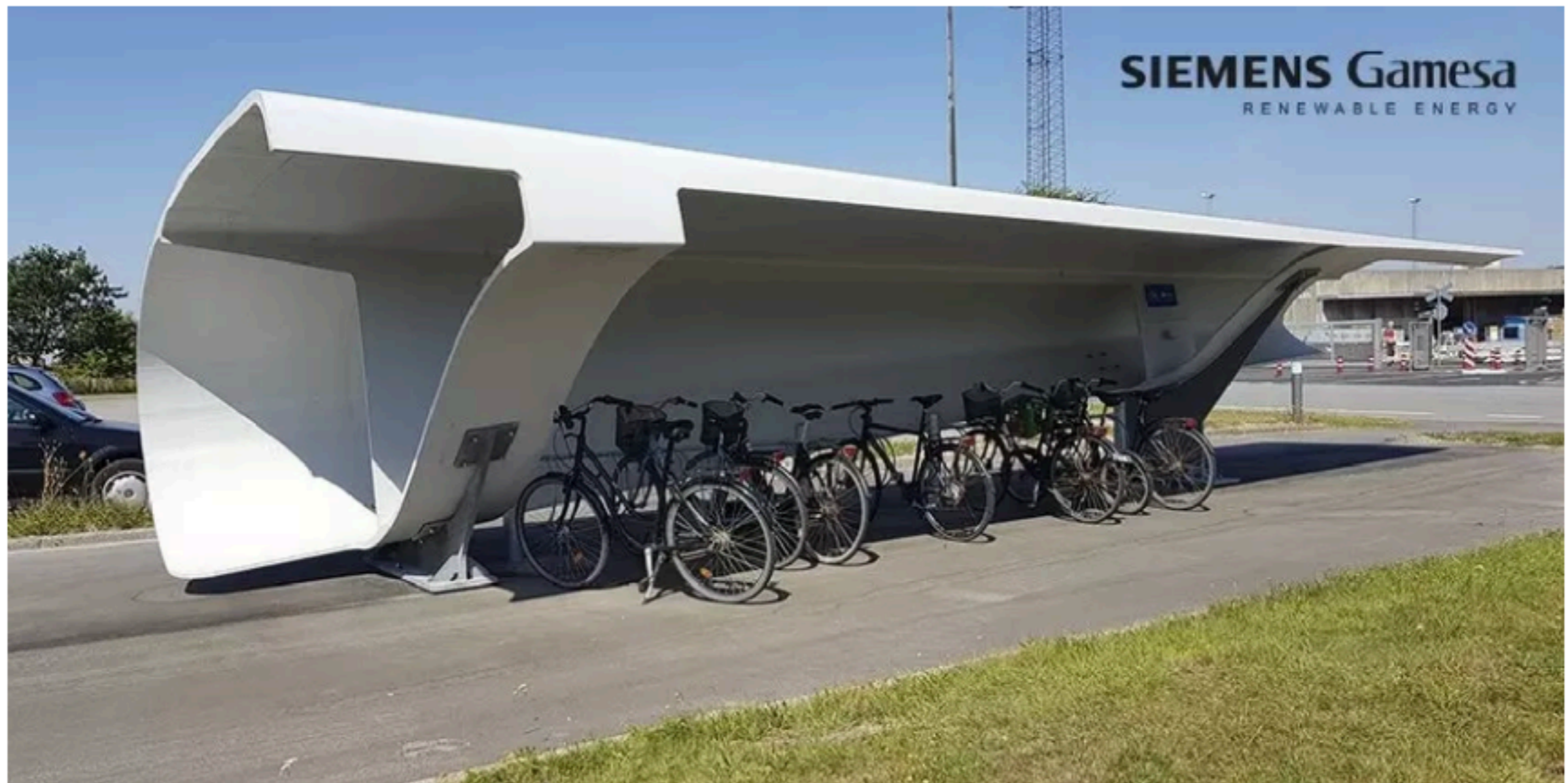
This image shows a section of turbine blade which shelters bikes in Denmark. Image: Siemens Gamesa via Twitter
