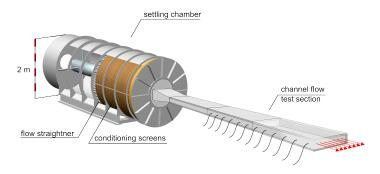
Abb.: Sketch of the wind tunnel.
